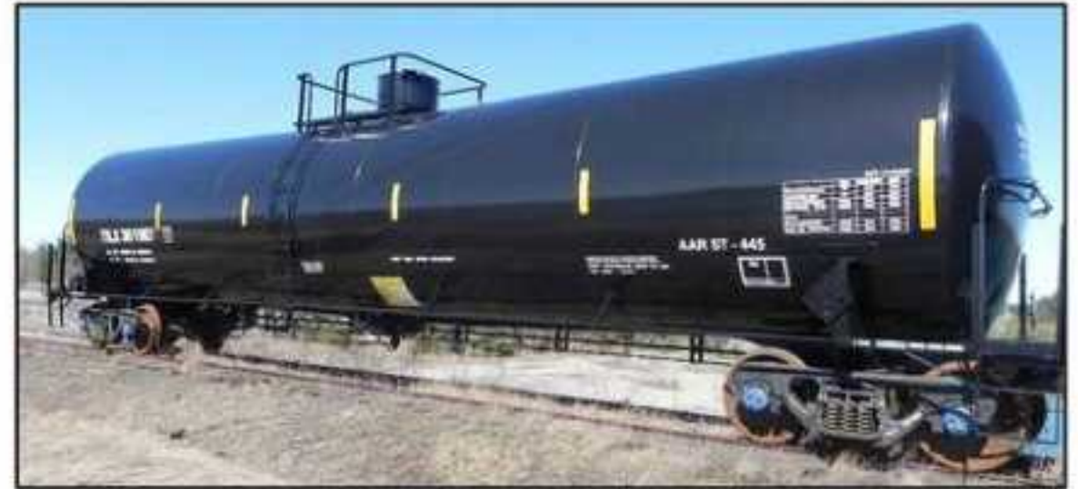
DOT/TC-117J100W Tank Car for Flammable Liquid Service
