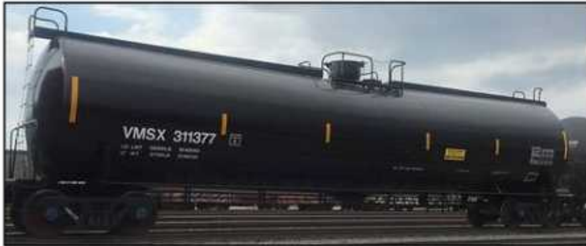
DOT/TC-117R100W Tank Car for Flammable Liquid Service
