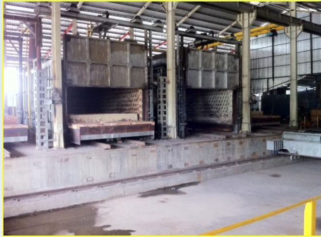
2 unit Heat Treatment 4x2x2m@6 ton 2 unit Heat Treatment 7x3.5x2.5m@20ton
