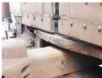
FIGURE A-2 EVIDENCE ON THE STRIKER OF COUPLER HORN CONTACT AND RUBBING
